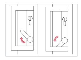
Note: the lock cannot be operated while the door is open due to the anti-slam device
